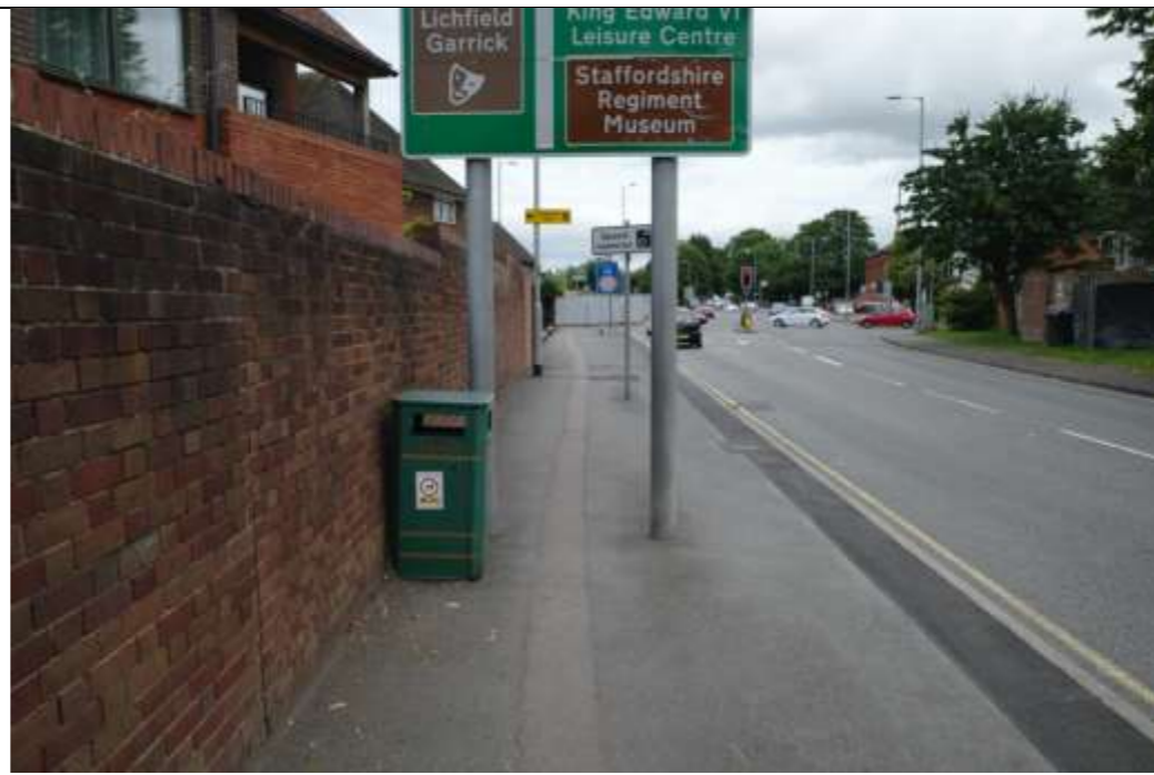
Signage intrusions into the footway on approach to junction with St John Street
