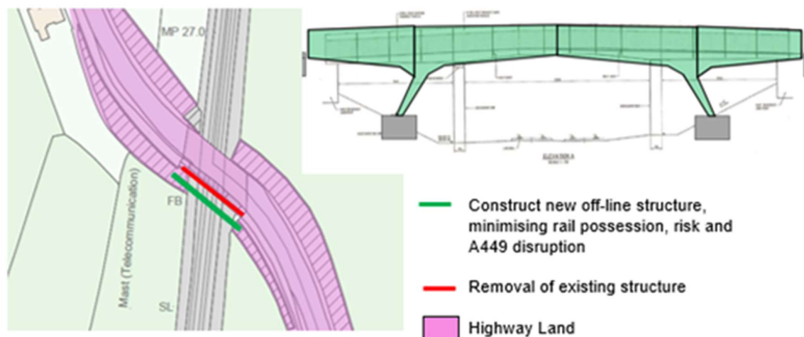
Figure 7 – Moss Pit Bridge Construction Drawing
