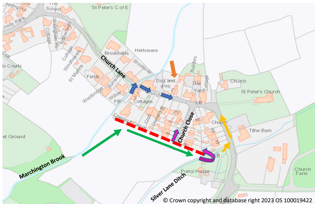
Figure 11: Observed flow routes at Church Lane, Marchington
