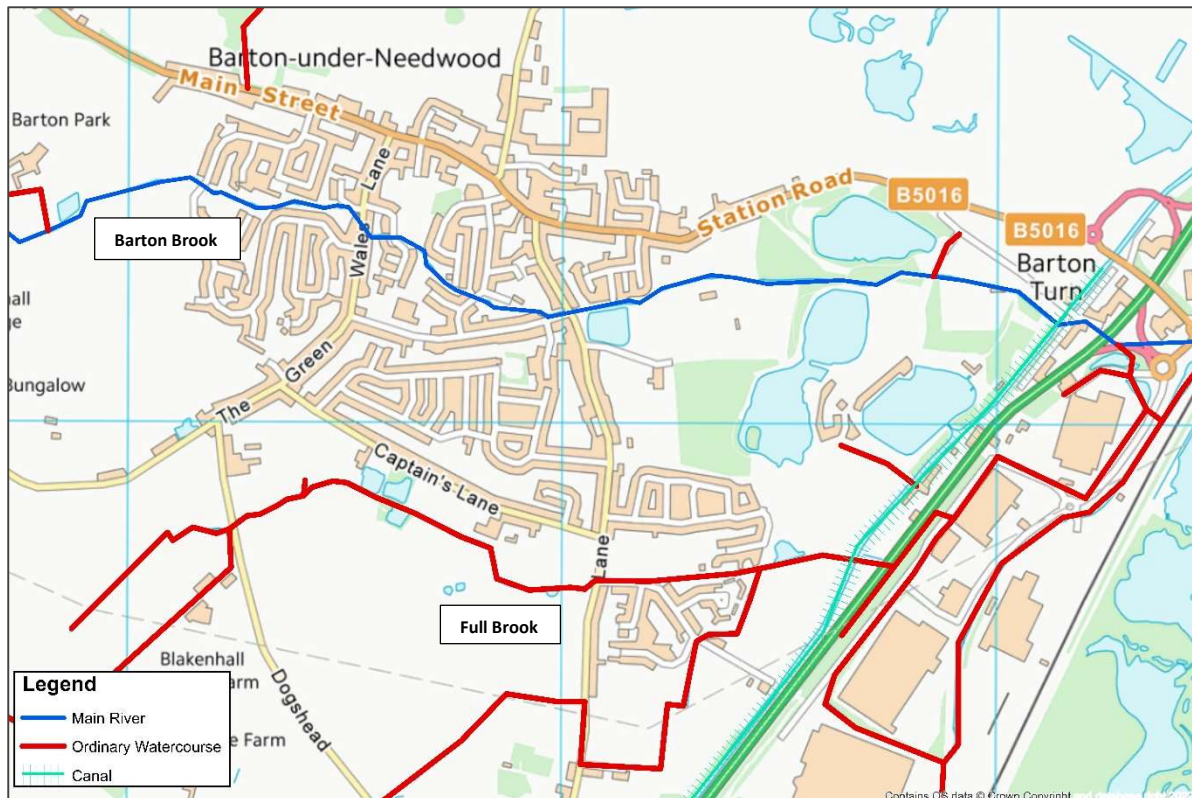
Figure 8: Watercourses discharging through and around Barton-under-Needwood that include the Barton Brook (main river) and the Full Brook (ordinary watercourse). This information is from the Detailed River Network (DRN) that may not include all present flow paths. This includes a discrepancy noted by the Barton Parish Council on the direction of the unnamed watercourse that joins the Full Brook, that has an additional direct flow path across land towards Mill Lane.
