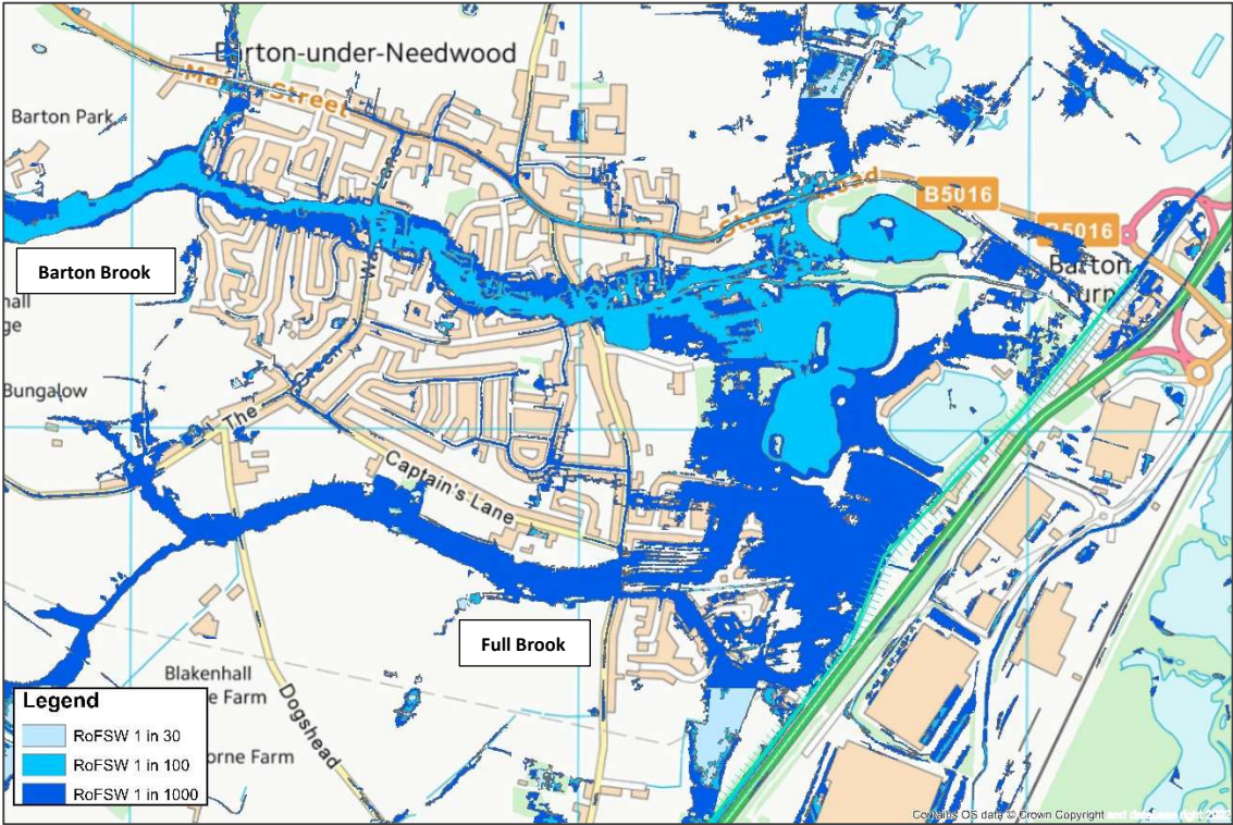
Figure 10: Environment Agency Risk of Flooding from Surface Water (RoFSW) map outlines (1 in 30 years, 1 in 100 years and 1 in 1000 years) for Barton-under-Needwood
