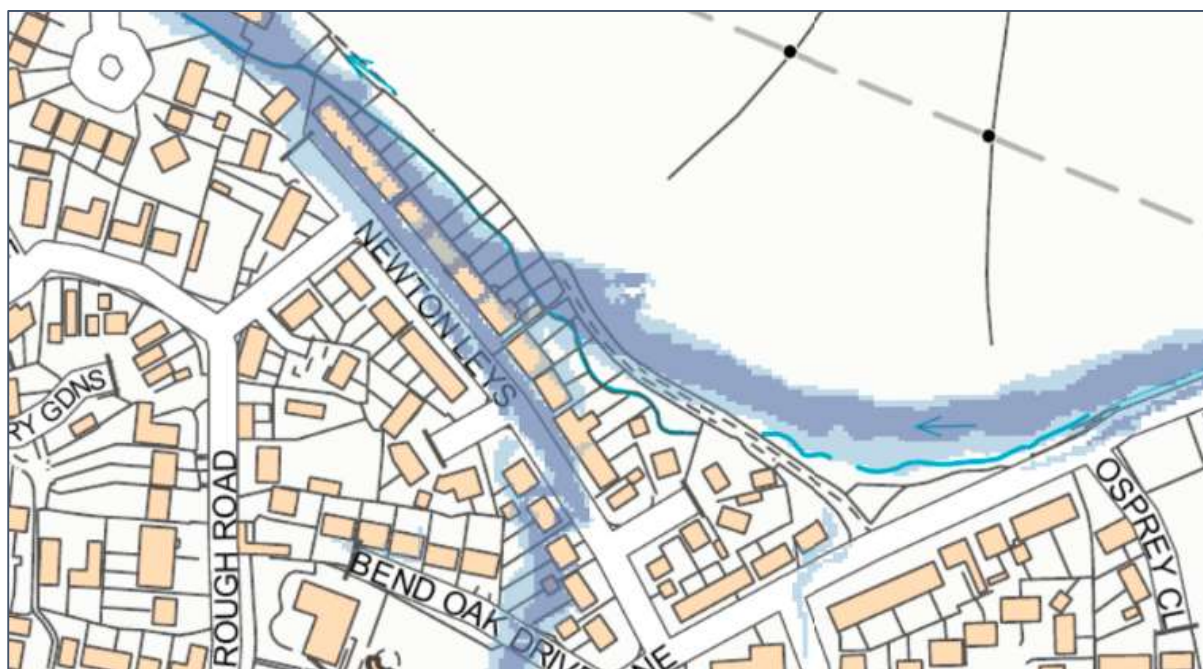
Figure 5: Newton Leys Location Plan with Risk of Flooding from Surface Waters Layers. RoFSW 1 in 30 years (Dark Blue), RoFSW 1 in 100 years (Light Blue)
