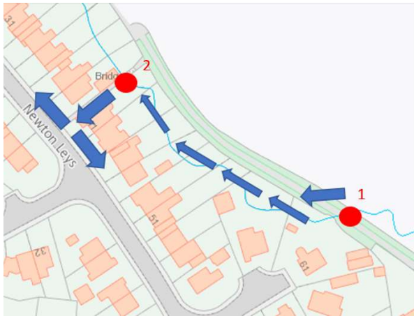
Figure 13 - Culverts (red circles) where footpaths cross the watercourse
